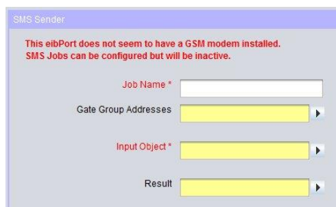
Figure 166: Job mask – GSM Modem not implemented / not detected
